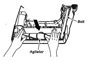
Check to see that the belt is centered on the belt pulley and that the agitator turns freely.
